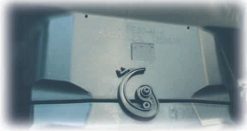
All plastics in a Scania vehicle are marked to facilitate sorting and recycling at the time of disassembly.
